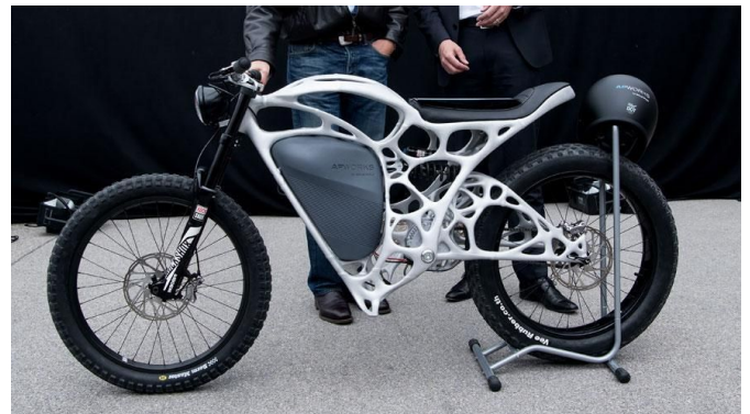
Figure 1: 3D-printed aluminum motorcycle [3]
