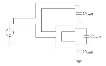
We divide the wires into 6 segments of fixed length  $l_i$ ; our variables will be the widths  $w_i$  of the segments. (The height of the wires is related to the particular IC technology process, and is fixed.) The total area used by the wires is, of course,
