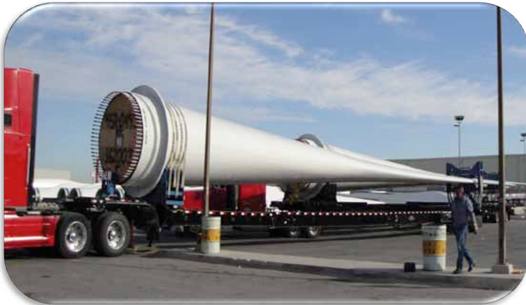
Current shipping configuration of 2.4MW 46.2m wind blade
