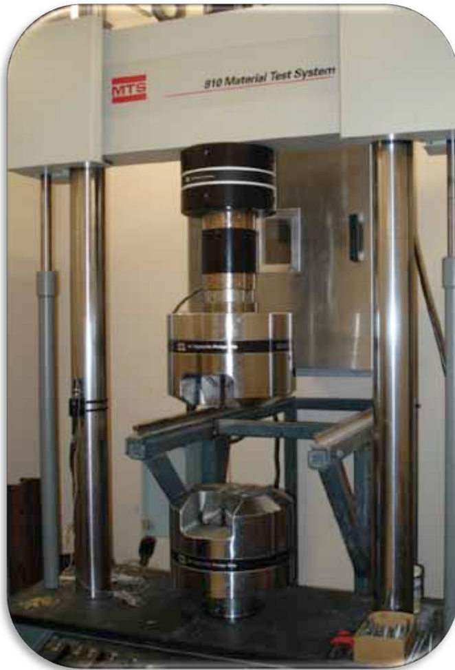
500kN Load Capacity with Environmental Chamber
