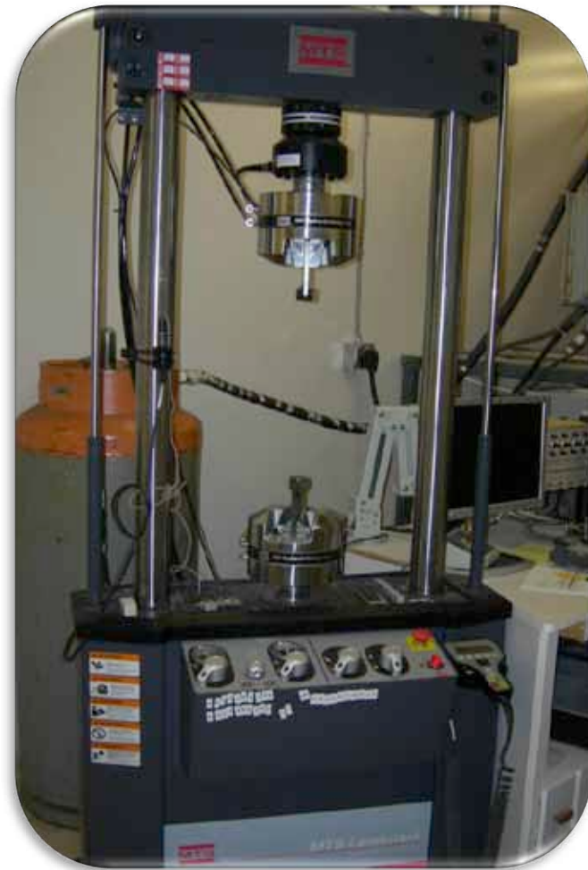
100kN Load Capacity for Resin testing and Cross-Plied Laminates
