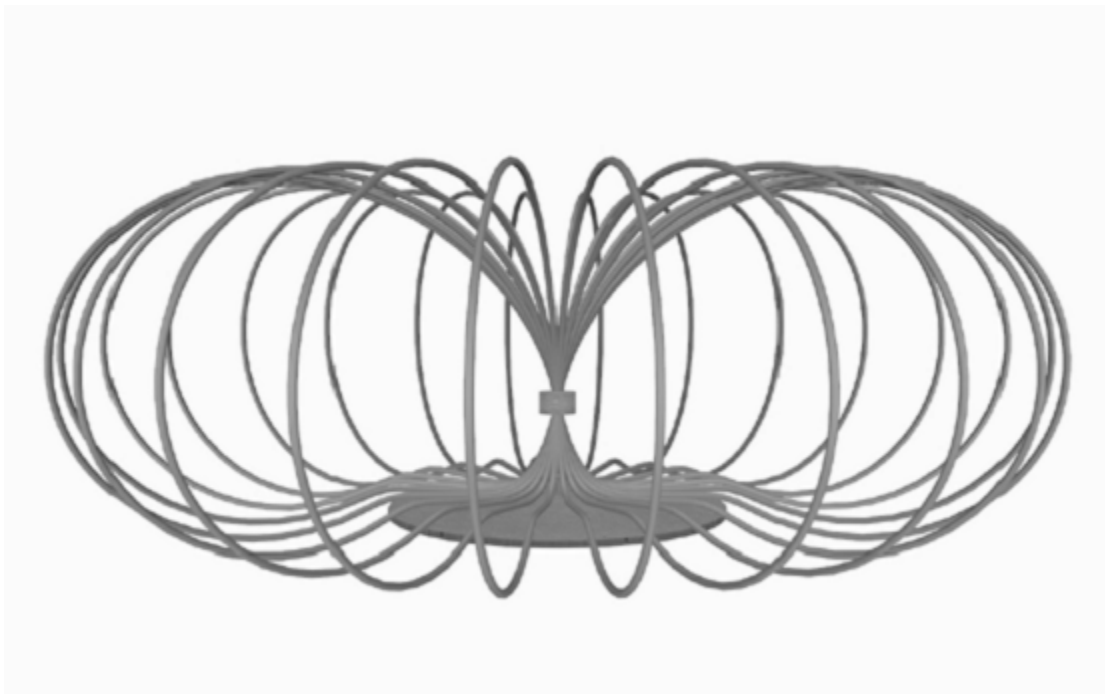
Figure 1.3-1: A magnet levitating above a disk with zero resistance.
