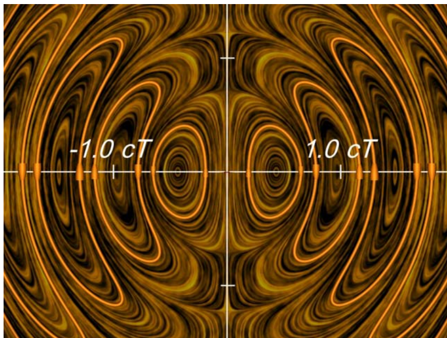
Figure 9-9: An oscillating dipole at the zero of the dipole moment, in the far zone
