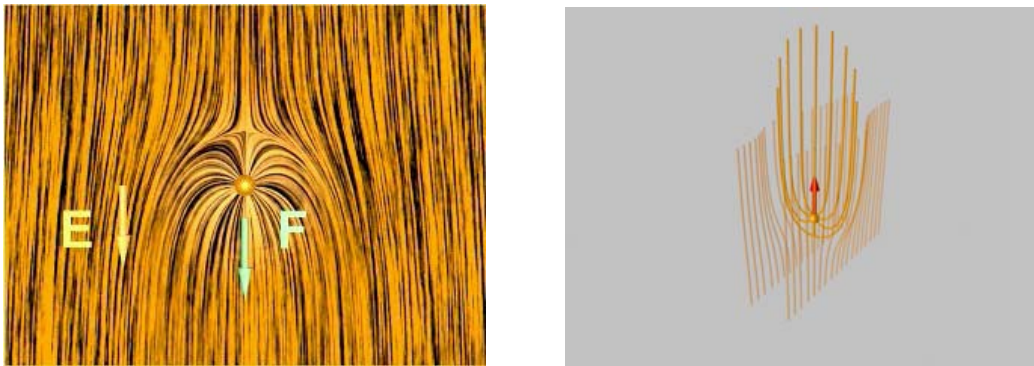
Figure 21-1: The q\mathbf{E} Force as Due to Maxwell Stresses and Tensions
