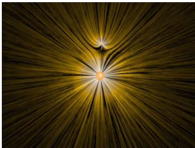
Figure 40: A positive charge moves past a massive positive particle at the origin and is deflected from its path by the stresses transmitted by the electric fields surrounding the charges.
