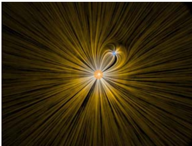
Figure 39: A negative charge moves past a massive positive particle at the origin and is deflected from its path by the stresses transmitted by the electric fields surrounding the charges.
