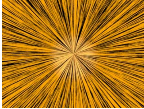
Figure 6: Representing the flow field associated with a source using textures.
