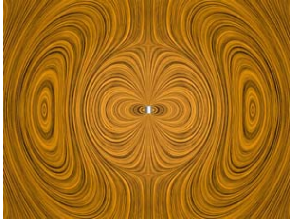
Figure 67: Electric dipole radiation from an electric dipole whose dipole moment completely reverses.
