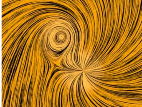
Figure 15: A fluid flow field that has both a source and a circulation.
