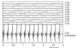
On the bottom we show the "raw" signal differentially recorded from a pair of leads at the occiput during continuous echo planar imaging (tr=3s, 19 slices, 128x64 matrix), with the ADC triggered to synchronize with the start of each tr. The traces above, in blue, show 10 sequentially acquired periods of EEG after subtracting the average of 30 EEG traces and are essentially free of contamination by the scanning artifact.
