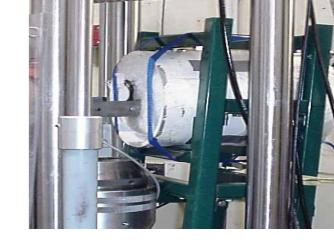
Pull to failure, two strain rates: 25 mm/s and 0.25 mm/sec
