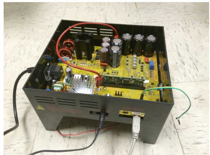
Fig. 9: Texas Instruments High Voltage 1 hp Motor Control Development Kit
