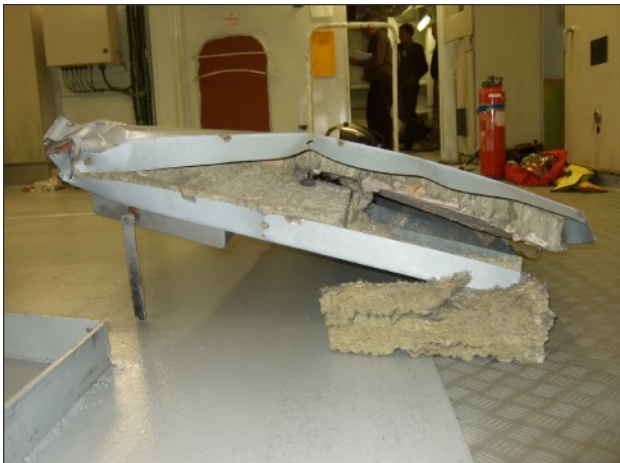
Fig. 18: Steel Door from Harmonic Filter Capacitor bank on Queen Mary II REF SB4-10
