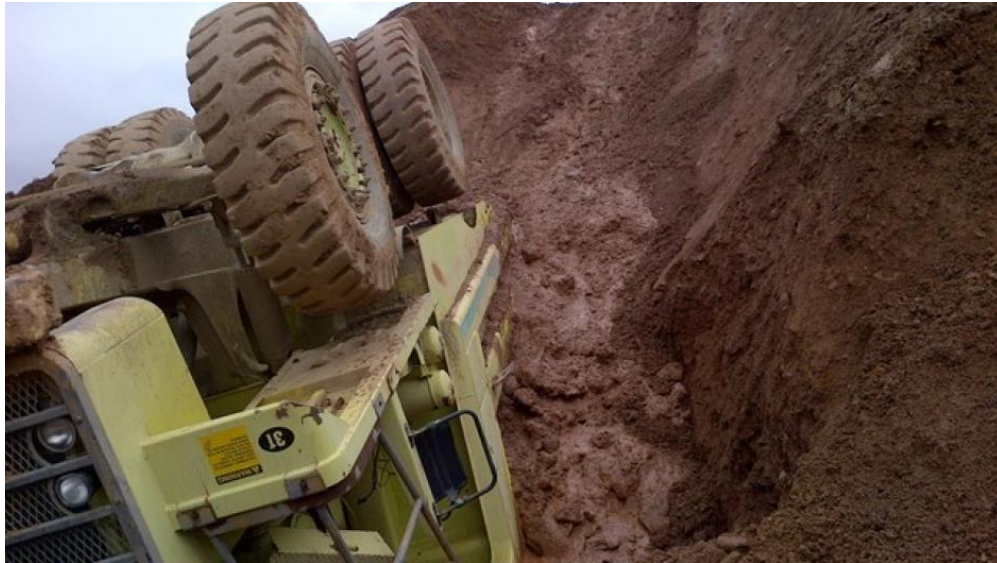
Figure 22 Haul truck overturned on dumpsite [61]
