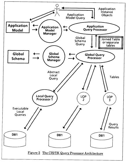
Central to the CIS/TK information processing capability is a query processor architecture as shown in Figure 2 [10, 11]. The architecture consists of an Application Query Processor (AQP), a Global Query Processor (GQP), and a Local Query Processor (LQP) to interface with the query command processor (e.g. a DBMS) for each database in the CIS.
