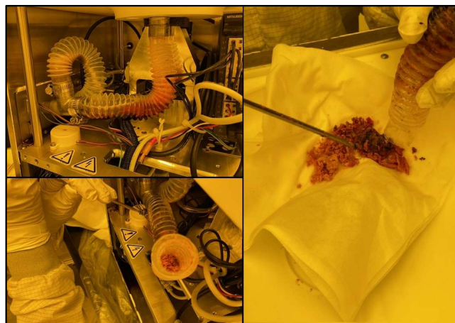
Fig. 1: Photographs showing a clogged spin-coater drain line. PMGI was mixed with acetone and precipitated, fully clogging the drain. This problem occurred in just a few weeks.
