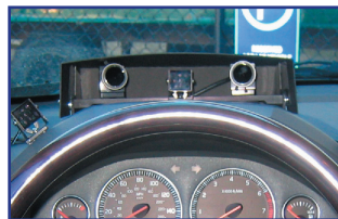
Fig. 3. Eye tracking system mounted on the dashboard
