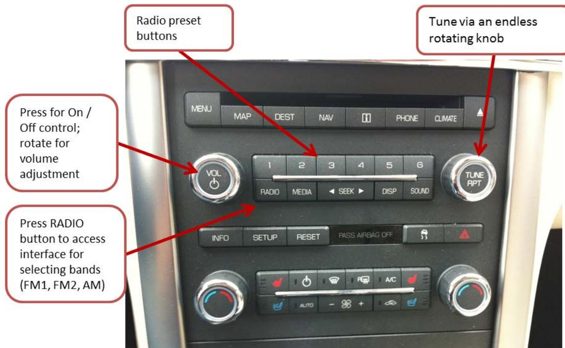
**Figure 5:** "Traditional" visual-manual radio interface in 2010 model year Lincoln MKS test vehicle. Switching between FM1, FM2, and AM radio bands was carried out using touch screen buttons on the main display screen located directly above the center console shown here.
