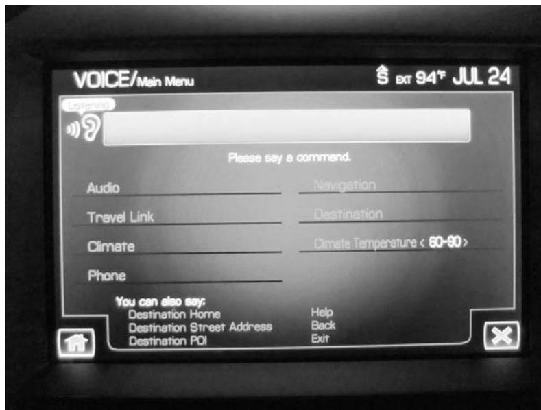
Figure 2: The screen above appears on the display screen at the top of the center console when the Push-to-Talk button is pressed.
