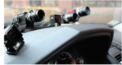
Machine vision cameras and a faceLAB eyetracking system keep a watchful eye on their subjects
