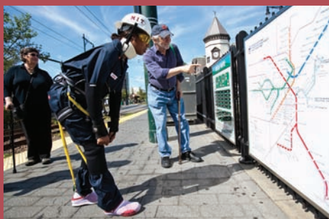
AGNES is designed to help product designers better understand the physical toils of old age
