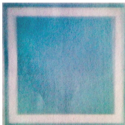
Fig. 7 Image of water soluble pentacene 4 ink-jet printed onto a flexible plastic substrate (Novole polyimide photopaper) using a DMSO based ink.
