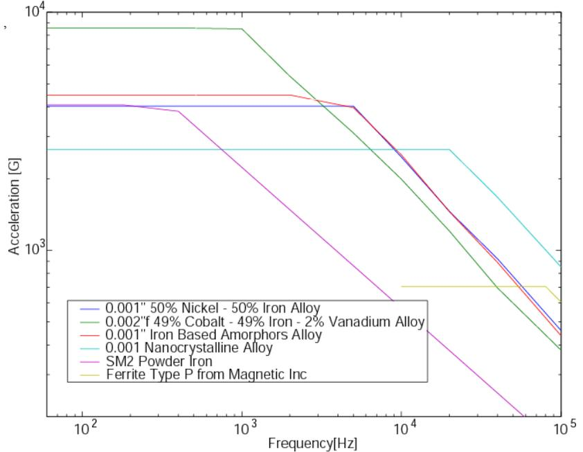
Fig 6. Typical soft magnetic materials acceleration performance. The energy loss is limited by  $0.25 \text{ W/cm}^3$ .
