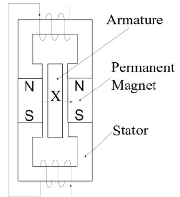
Fig 2. A hybrid fast motor
