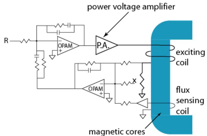
Fig 7. Power amplifier control circuit with flux feedback..
