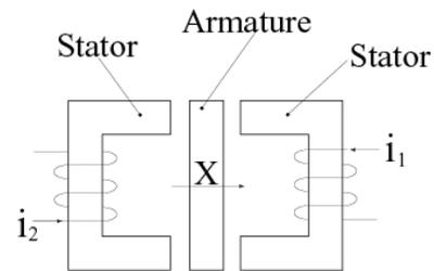
Fig 1. Solenoid-type fast motor
