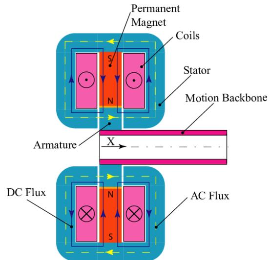
Fig 3. Ultra-fast motor working principle
