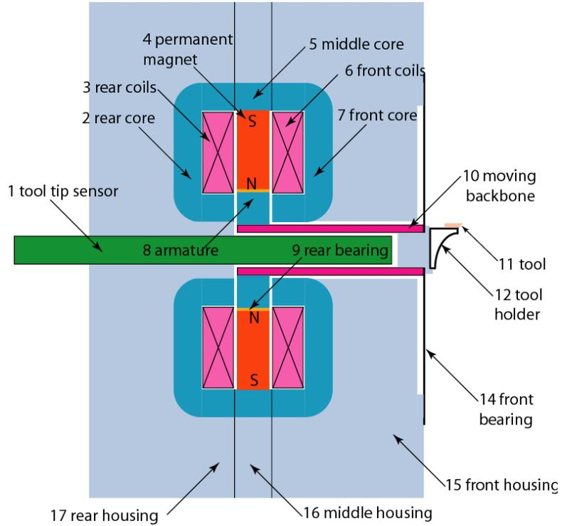
Fig 5 Linear ultra fast tool servo design details.
