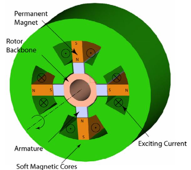
Fig 4. Rotary ultra-fast motor concept.
