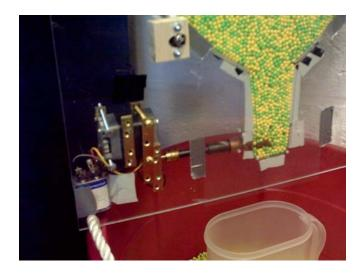
Figure 20: Motor and Drill Removal Device
