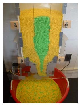
Figure 25: Annulus Behavior Near End of Drain Down
