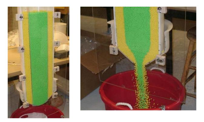
Figure 12: Continuous Flow Experiment with Dynamic Central Column
