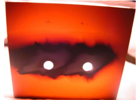
Light transmission through SiC mask and sample
