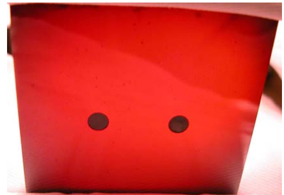
Light transmission through SiC mask and sample
