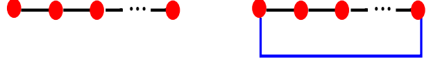
Fig. 2. Comparison of a network with open chain structure and another one as a closed ring.
