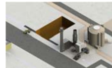
(A) Excavation occurs adjacent to an existing Mk1 unit, with protected area fence rerouted
