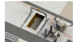
(B) Basemat is poured after common tunnel and lift-tower have been installed
