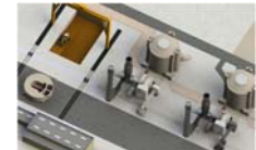
(D) After above-grade modules are installed, fence is rerouted before loading fuel
