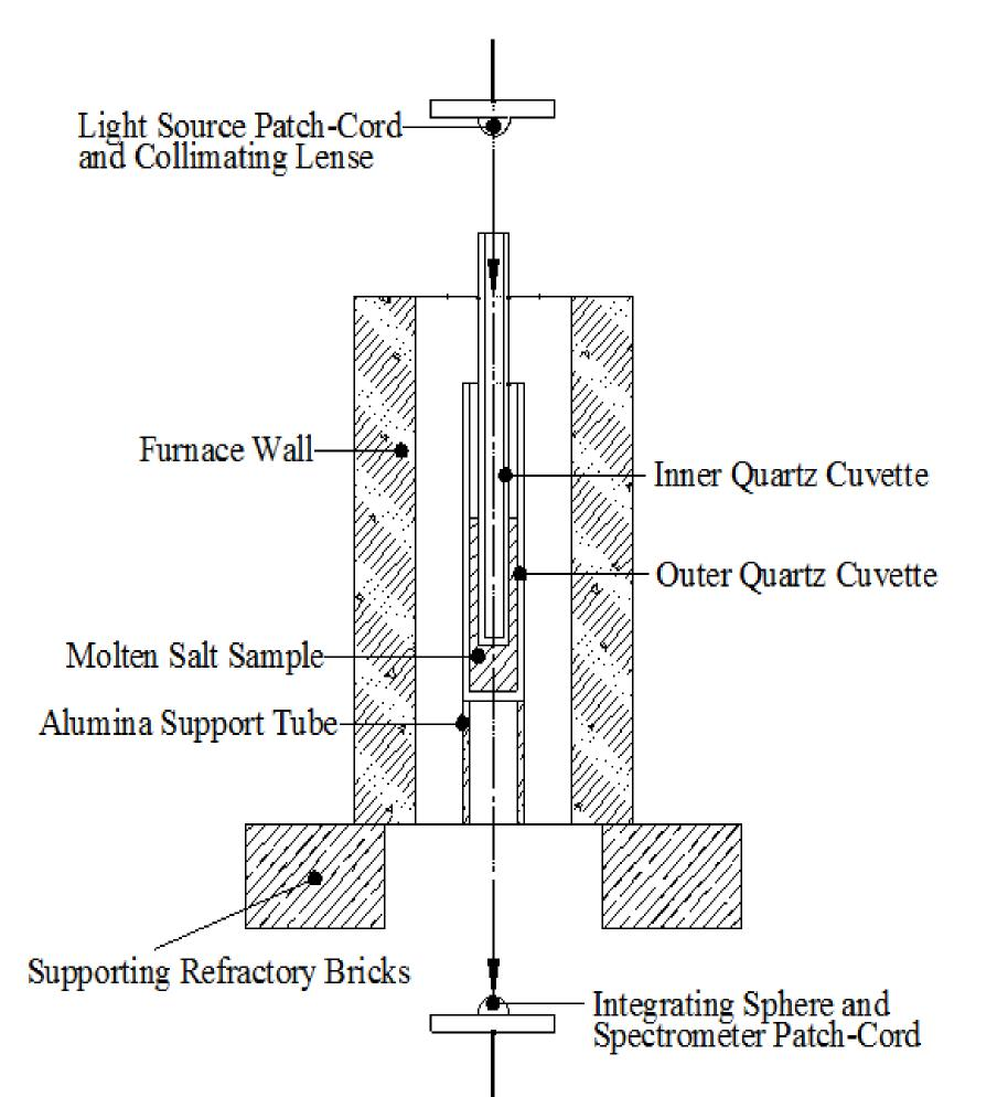
Goal: Use a custom built experimental apparatus to measure absorption of light with temperature and wavelength.
