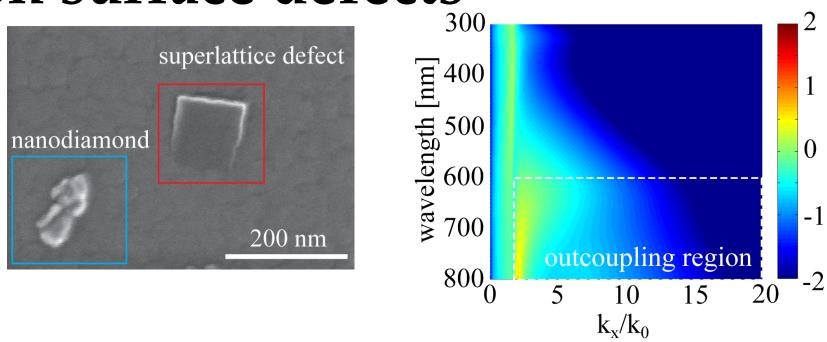
Superlattice defects with the size of ~50 nm can scatter into far-field the high-k modes with  $k_x/k_0 \sim 20$ . In FEM simulations, we showed that due to these defects on HMM the collected emission can be increased further.
