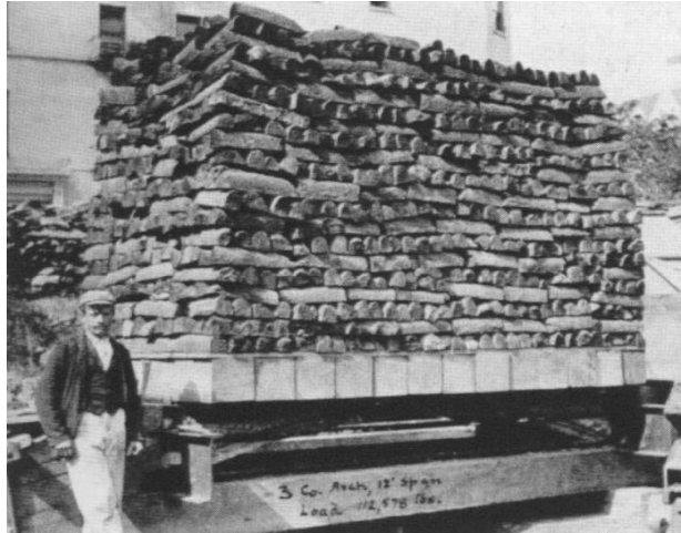
Figure 4. Strength test of a 12 ft span timbrel vault, three courses thick, supporting a load of 112,578 lbs of pig iron (23 May 1901) (Tarragó, 2002).
