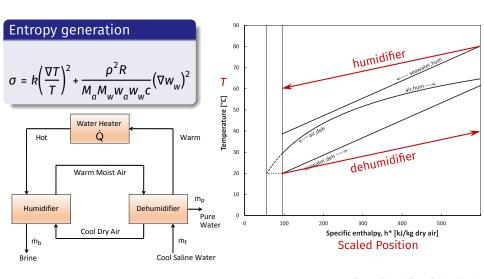
Entropy generation minimization thru balancing: HCR<sub>d</sub> = 1
