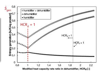
Energy efficiency maximized at HCR of minimum entropy generation
