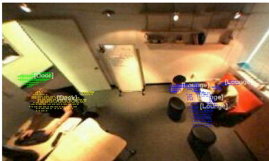
Fig. 10. The workspace overlaid with clustered tracker data for three different zones; zone labels (door, desk, lounge) are user-supplied
