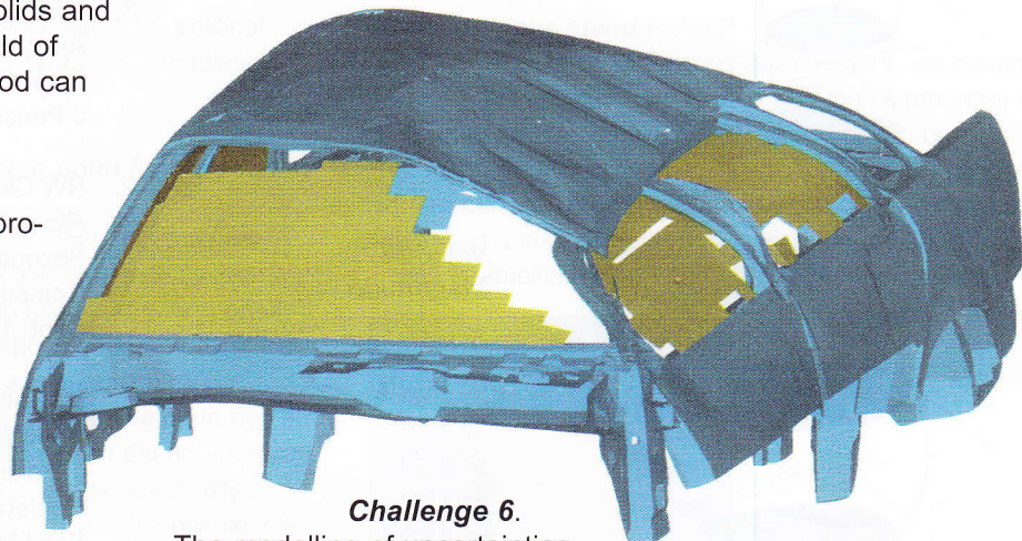
Figure 3: Crushing of a motor car model
