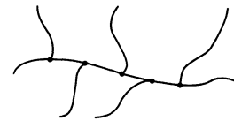
Fig. 4.5. — The topology of comb polymers. There are g branch points and g + 2 linear chains.
