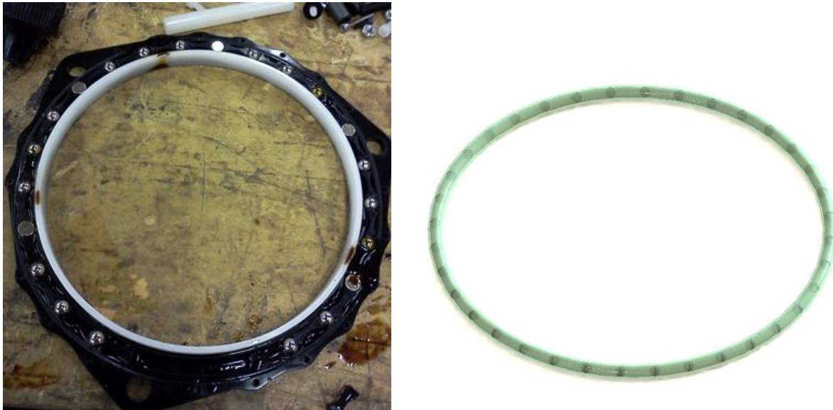
Figure 3-7. Damper Detail. Showing the inside of the old damper design as well as a solid rendering of the new simpler design which uses a prebuilt plastic tube.
