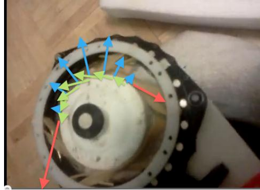
Figure 4-2. Showing the model of the interaction between the elastic encircling elements and the object being gripped. Figure 2. Red arrow shows tension force, Blue shows normal force (On the bottle) and green shows the frictional forces, which combine to create the torque on the object.
