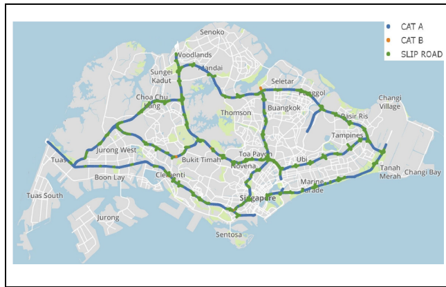
Figure 2. Singapore road network consisting of 2,139 highways, 10 arterial, and 747 slip roads.
