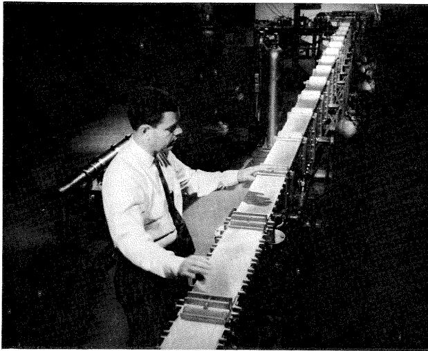
17. Shock tube for producing moving normal shock waves in the laboratory.
