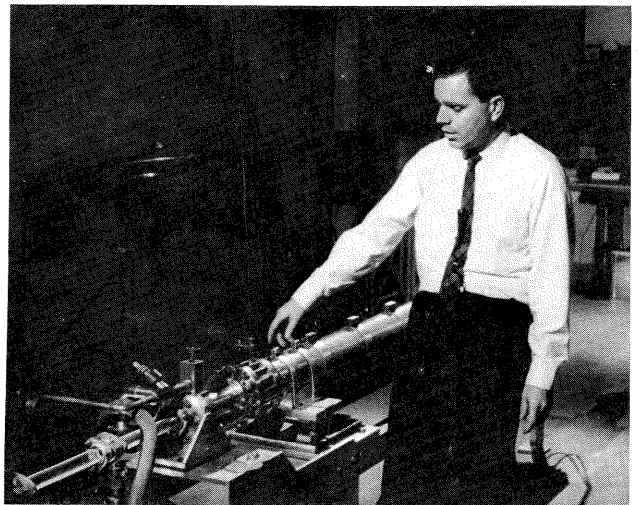
20. Shock tube for producing very strong normal shock waves.
