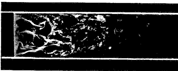
1. Channel flow visualized by hydrogen bubbles released uniformly from a wire stretched across the flow.
