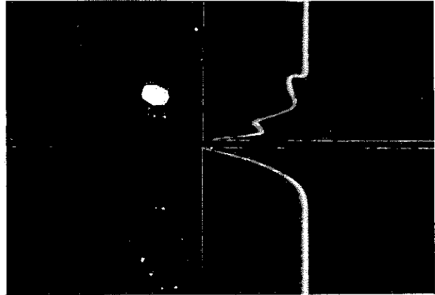
19. Instantaneous displacement profiles for flow along a thin plate. The boundary layer on the upper surface has been made turbulent, while the flow along the lower surface is laminar.
