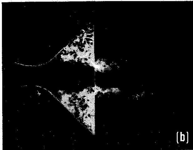
8. Hydrogen bubbles mark the flow in a diffuser. Flow is from left to right. (a) Small divergence angle. The flow remains attached. (b) Large divergence angle. The flow detaches.
