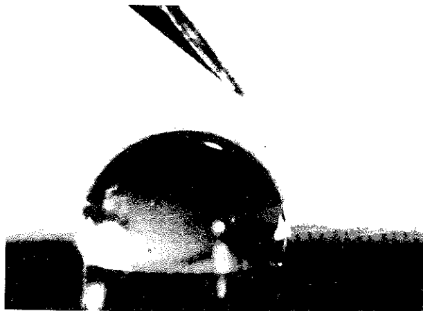
3. A drop of water placed on wax by means of a hypodermic needle demonstrates a liquid angle greater than 90^\circ . Water does not wet wax.
