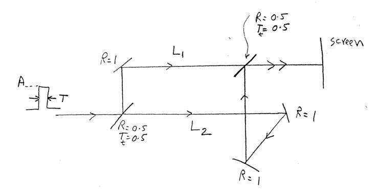
If the input to the interferometer shown in the figure is a pulse of amplitude A=1 watt, and width T=1 nanosecond, sketch the intensity you would observe on the screen as a function of pathlength difference  $(L_2-L_1)$  from 0 to 50 cm. Comment on your observations.
