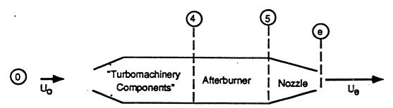
Turbojet can be run with afterburner off (exit temperature =  $T_{t_e}$ ), or on (exit temperature =  $T_{t_e}$  =  $2T_{t_e}$ )
