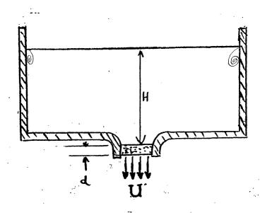
A container filled with water to a level H is fitted with a spout containing a porous plug through which the water empties. The resistance of the plug may be expressed by the formula
