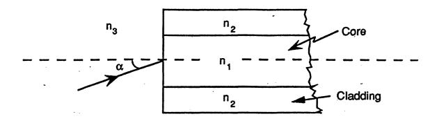
The figure shows a 2-dimensional optical fiber or waveguide. The index of the core is  $n_1$  and the index of the cladding is  $n_2$ , where  $n_1 > n_2$ . A ray of light entering the core from the outside at an angle of incidence,  $\alpha$ , as shown, will propagate without loss via a series of total internal reflections at the core-cladding interface, as long as  $\alpha$  is below a certain value.
