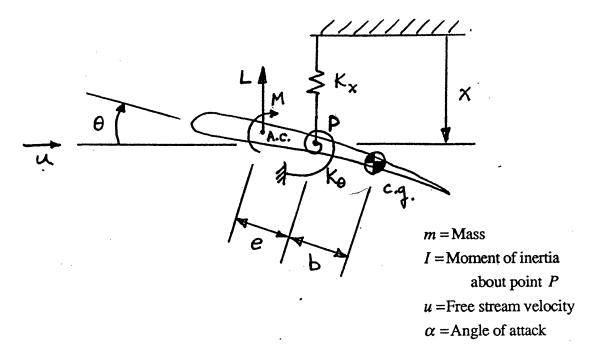
The straight wing section above is placed into a wind tunnel to study its flutter behavior. It is free to move vertically (x) and in pitch  $(\theta)$  about point P, with springs attached to each degree of freedom  $(K_x \& K_\theta)$ . In addition, the aerodynamic forces can be approximated as:
