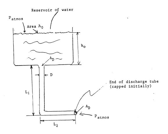
Consider a large reservoir of water, as shown, open to the atmosphere. The open surface has area  $A_0$ , the reservoir has vertical sides, and the initial depth is  $h_0$ .
