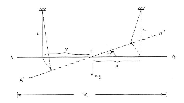
A thin, rigid rod of length, R, and mass, m, is suspended by two vertical strings of length, L, each separated from the bar's center of mass, C, by a distance, D. Obtain the differential equation of motion for small rotations,  $\Theta$ , of the bar in the horizontal about a vertical axis through C. Determine the period of the oscillation and describe how the period would change as the distance, D, is decreased toward zero.
