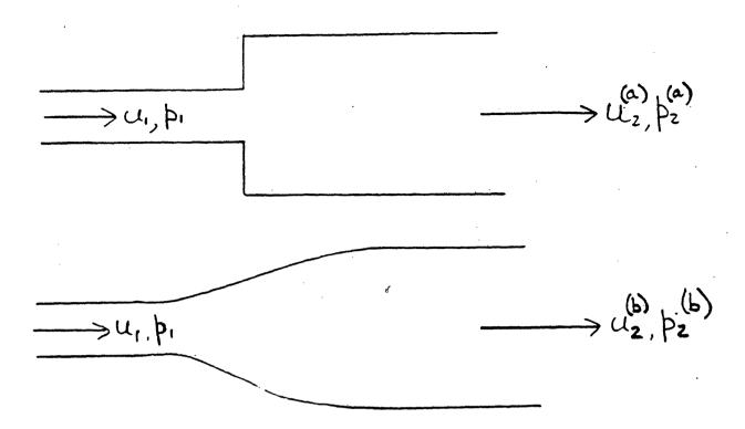
Consider the flow of an incompressible fluid in the junction between two pipes of cross-sectional area  $A_1$  and  $A_2$ . Assuming that the Reynolds number is large, discuss the different qualitative nature of the flow in an abrupt and a smooth junction (pictured above). Explaining any approximations clearly, derive equations for the outflow variables  $u_2$ ,  $p_2$  in the two cases.
