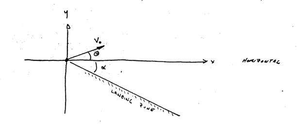
An olympic ski jumper leaves the origin of coordinates at time zero with a velocity magnitude,  $V_0$ , and free-falls to a landing on a flat surface that is inclined to the horizontal by an angle  $\alpha$ . What angle,  $\theta$ , should his initial velocity make with the horizontal to achieve the maximum length jump? What horizontal distance will he cover if he uses the optimum  $\theta$ ?
