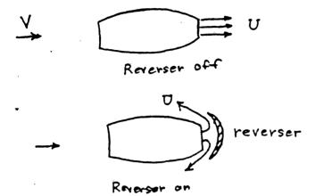
shown shematically at the left. If the reverser turns the flow through an angle of 135° without appreciably altering the relative exit speed flow, U, if the forward speed of the engine is V and the engine massflow is m, what is the change in thrust between operation with reverser off and reverser on?
