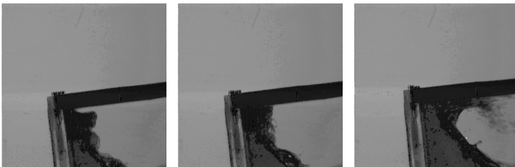
Fig.8 Occurrence of tank-top impact and formation of splashes: SNU model, 50% filling
