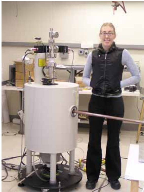
Melissa Hornstein and her 460 GHz gyrotron oscillator
