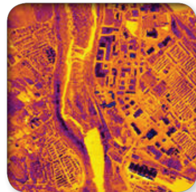
Figure 3. Thermal mapping in England demonstrates which roofs loose the most heat to the atmosphere, an indicator of the insulation capacity of the roof. http://www.bluesky-world.com/products/
