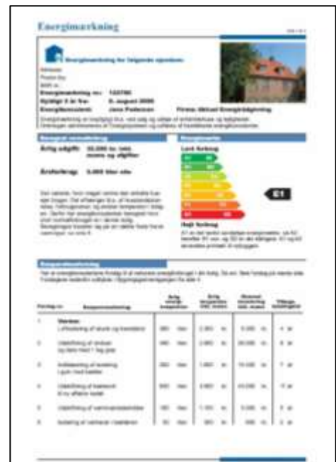
Figure 1: A Danish building energy label, which includes a letter grade from A-G, key energy use metrics, and the assessor name. Source: BuildingRating.org 2011.
