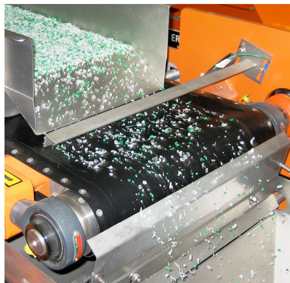
Fig. 7. Rare-earth magnetic roller process.
