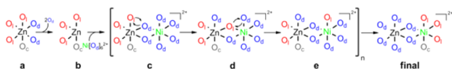
Figure 3. Schematic representation for the initial steps of the replacement of one O_d on Ni by O_l in the associative mechanism of the transmetalation of MOF-5. Reiteration of steps c–e yields the final lattice Ni-MOF-5. Only the substituted Zn, the incoming Ni, and their surrounding oxygens are shown for the sake of clarity. Oxygen atom label code: O_l , from the linker; O_d , from DMF; O_c , from the Zn_4O core.
