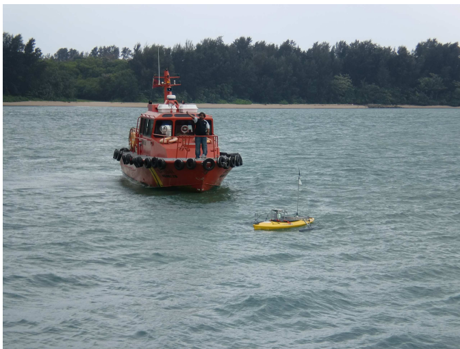
Fig. 10. ASC with the Velodyne 3D Laser during the experiment. The safety boat seen in the background was also considered as a feature during the experiment.
