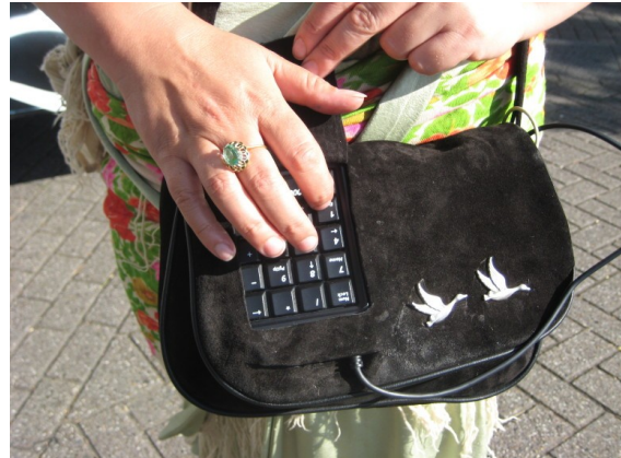
Fig:1,2# operating auto script with number keypad, bag in action recording and streaming audio/ uploading .jpgs to the server.
