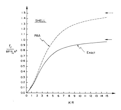
FIG. 5. The reduced rotatory friction coefficient for the shell versus  $(\kappa R)$  according to the mean field (-) and PAA (--) theories. The asymptotic values for large  $(\kappa R)$  are indicated by arrows.
