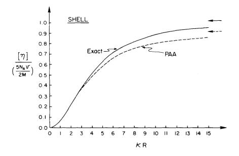
FIG. 3. The reduced intrinsic viscosity for the shell versus  $(\kappa R)$  according to the mean field (—) and PAA(——) theories. The asymptotic values for large  $(\kappa R)$  are indicated by arrows).
