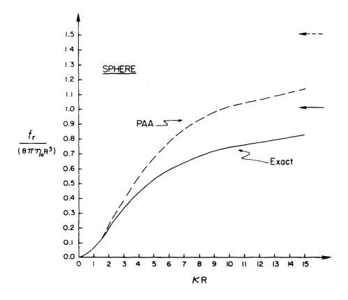
FIG. 4. The reduced rotatory friction coefficient for the sphere versus  $(\kappa R)$  according to the mean field (-) and PAA (--) theories. The asymptotic values for large  $(\kappa R)$  are indicated by arrows.
