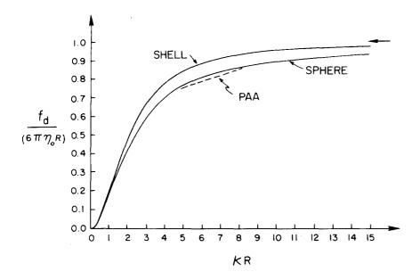
FIG. 1. The reduced translational friction coefficient for the sphere and the shell versus  $(\kappa R)$ . For the shell the mean field and PAA theories give identical results. For the sphere, the minor difference between the mean field and PAA theories are exaggerated.
