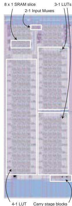
Figure 12: Layout of the computational cell.
